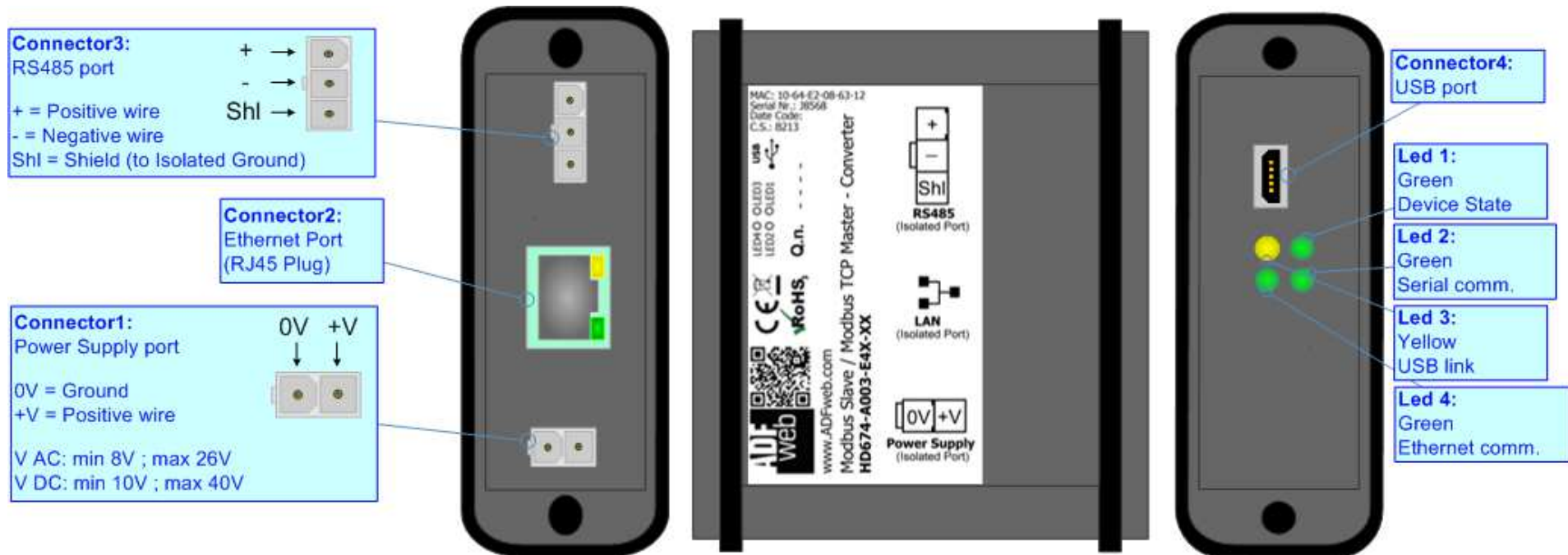
Figure 1a: Connection scheme for HD674-A003-E4x-xx
