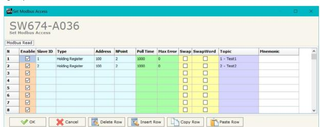
Figure 6: "Set Access → Modbus Read"
