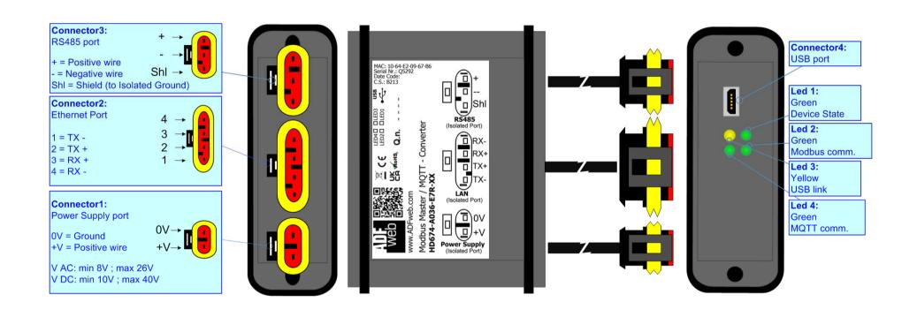
Figure 1b: Connection scheme for HD674-A036-E7x-xx
