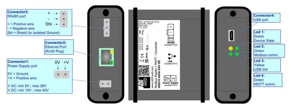
Figure 1a: Connection scheme for HD674-A036-E4x-xx
