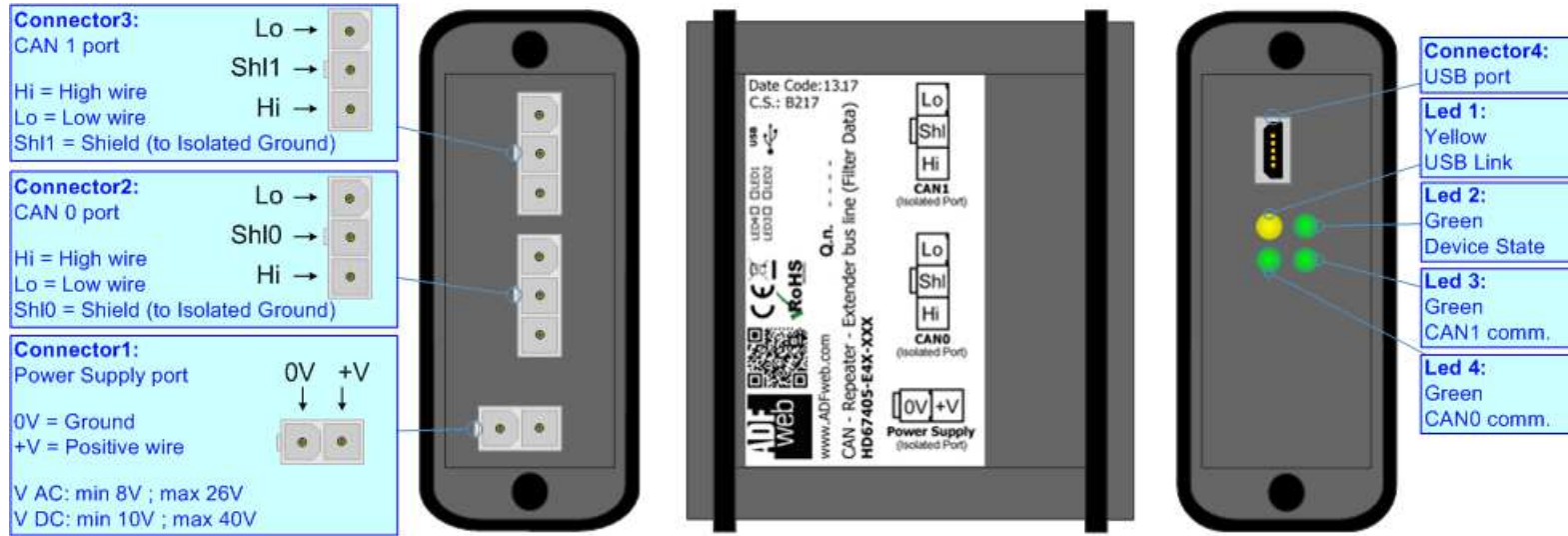
Figure 1a: Connection scheme for HD67405-E4x-xxx
