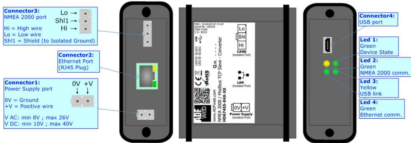
Figure 1a: Connection scheme for HD67455-E4x-xx
