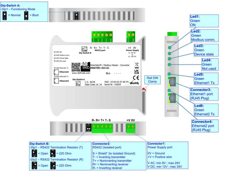
Figure 1c: Connection scheme for HD67591-422-A1
