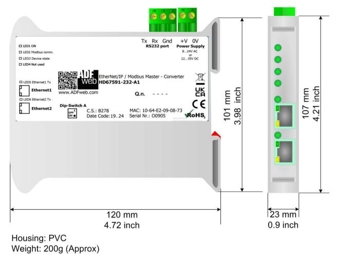
Figure 7a: Mechanical dimensions scheme for HD67591-232-A1
