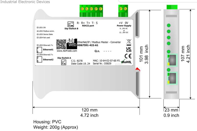
Figure 7c: Mechanical dimensions scheme for HD67591-422-A1
