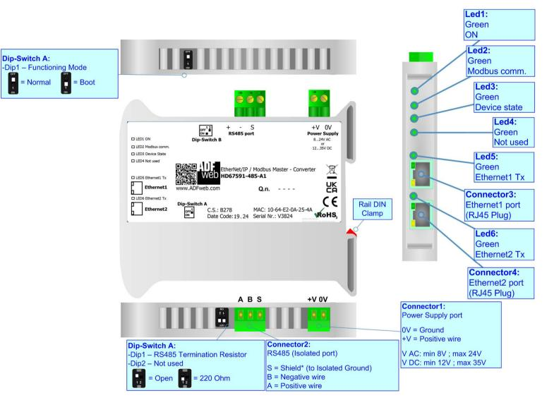
Figure 1b: Connection scheme for HD67591-485-A1
