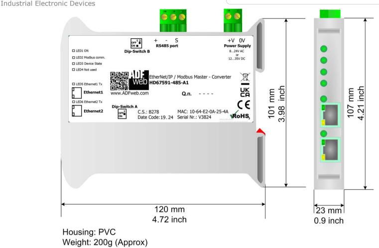
Figure 7b: Mechanical dimensions scheme for HD67591-485-A1
