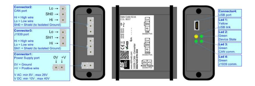
Figure 1a: Connection scheme for HD67439-E4x-xxx
