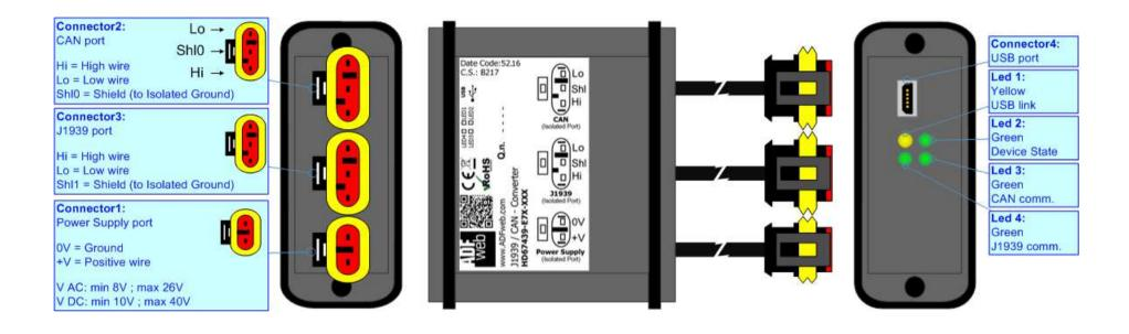
Figure 1b: Connection scheme for HD67439-E7x-xxx
