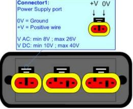
Note: It is possible to use also negative tensions. In this case the polarity must be inverted.
