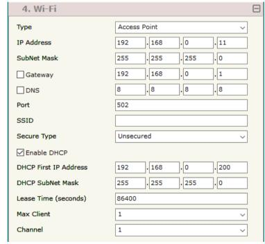
Figure 3e: "Set Communication → Wi-Fi" window
