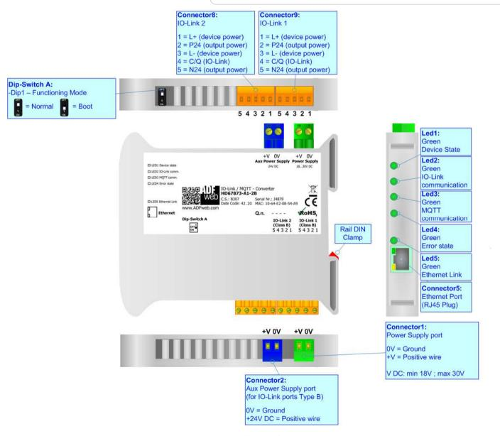
Figure 1c: Connection scheme for HD67873-A1-2B
