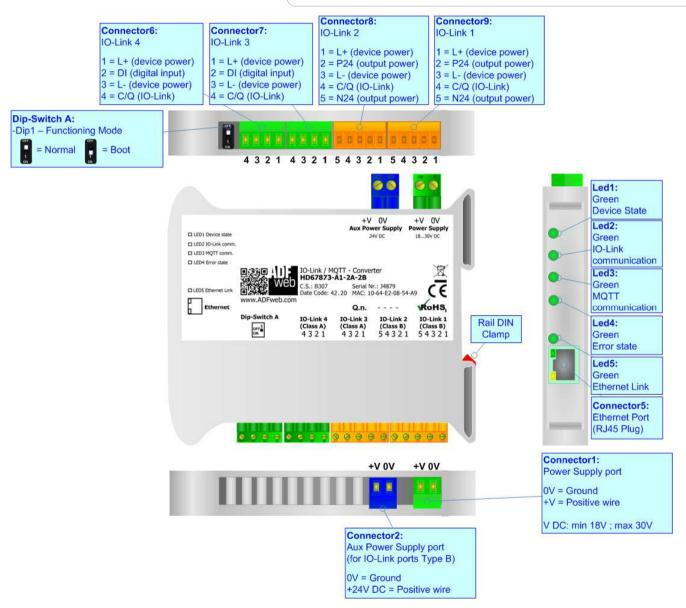
Figure 1d: Connection scheme for HD67873-A1-2A-2B
