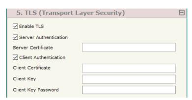
Figure 3q: "Set Communication → TLS" window
