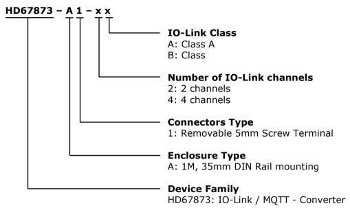
Order Code: **HD67873-A1-2A** - IO-Link / MQTT - Converter (IO-Link ports: 2 x Class A)
