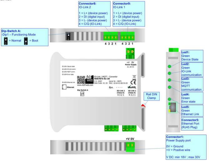
Figure 1a: Connection scheme for HD67873-A1-2A
