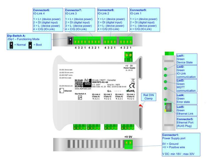
Figure 1b: Connection scheme for HD67873-A1-4A
