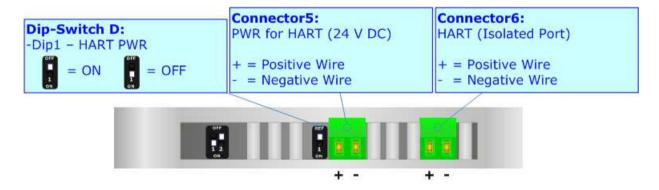
It is possible to provide the current loop for HART communication and an additional low power supply @ 24 V DC for feeding HART devices by setting Dip-Switch D at ON position.
