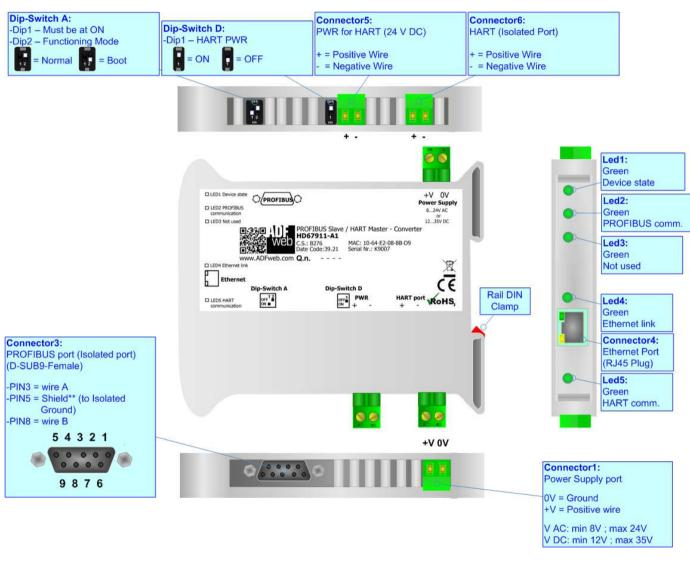
Figure 1: Connection scheme for HD67911-A1
