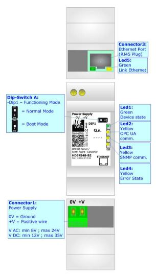
Figure 1: Connection scheme for HD67B48-B2
