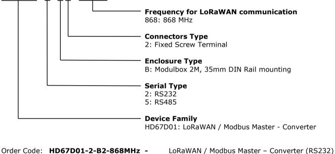
Order Code: HD67D01-5-B2-868MHz - LoRaWAN / Modbus Master – Converter (RS485)
