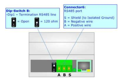
The maximum length of the cable should be 1200m (4000 feet).
