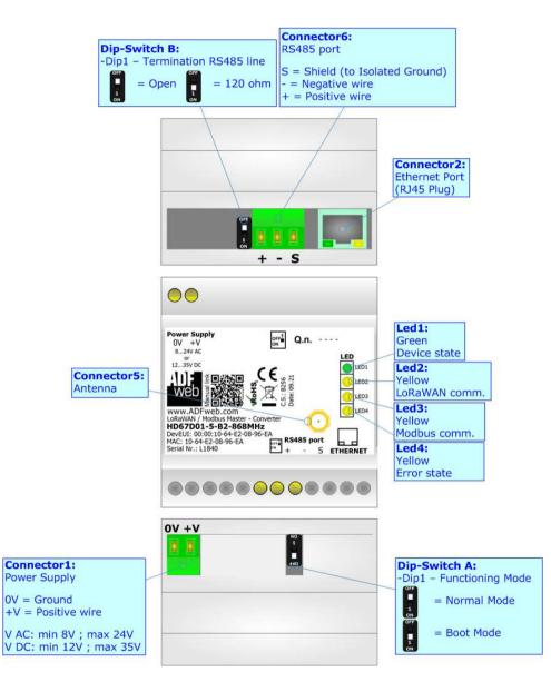
Figure 1b: Connection scheme for HD67D01-5-B2-xxxMHz
