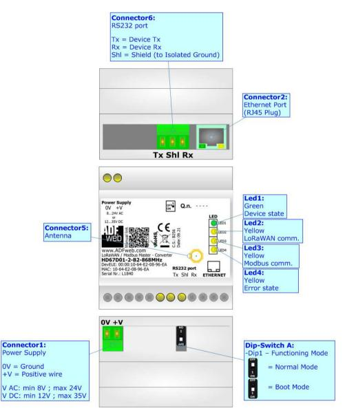
Figure 1a: Connection scheme for HD67D01-2-B2-xxxMHz
