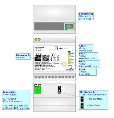
Figure 1: Connection scheme for HD67D24-B2-xxxMHz
