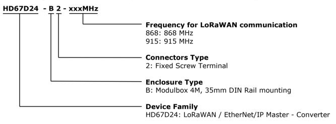
Order Code: **HD67D24-B2-868MHz** - LoRaWAN / EtherNet/IP Master - Converter Code: **HD67D24-B2-915MHz** - LoRaWAN / EtherNet/IP Master - Converter
