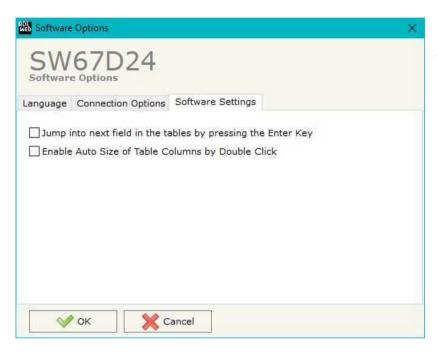
In the section "Software Settings", it is possible to enable/disable some keyboard's commands for an easier navigation inside the tables contained in the different sections of the software.
