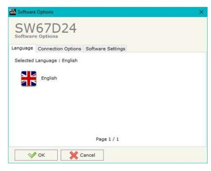
In the section "Connection Options", it is possible to check if there are some updatings of the software compositor in ADFweb.com website. Checking the option "Check Software Update at Start of Program", the SW67D24 check automatically if there are updatings when it is launched.
