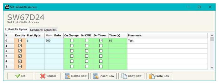
Figure 4a: "LoRaWAN Access → LoRaWAN Uplink" window
