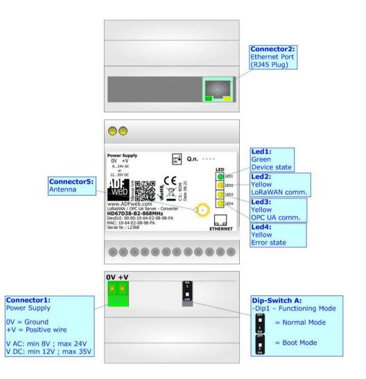
Figure 1: Connection scheme for HD67D38-B2-xxxMHz
