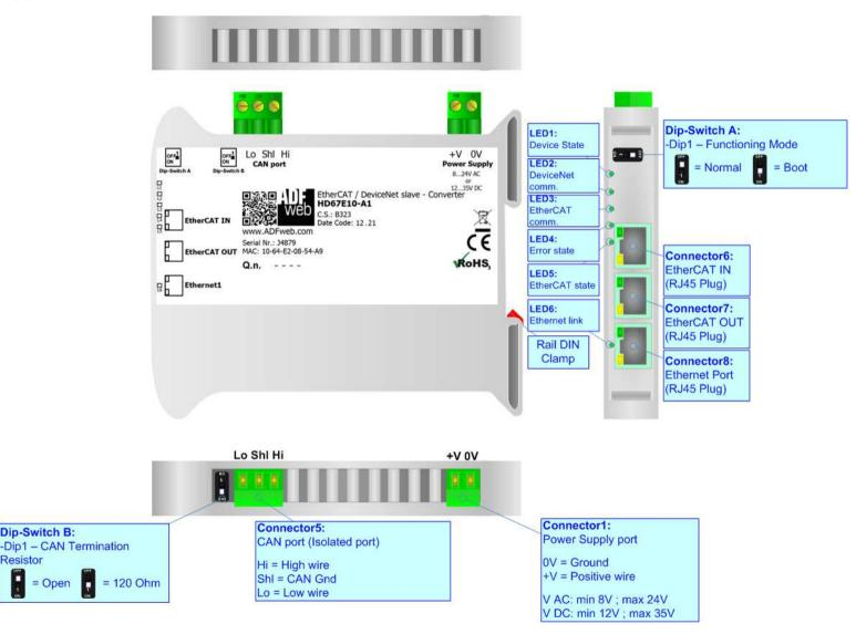
Figure 1: Connection scheme for HD67E10-A1
