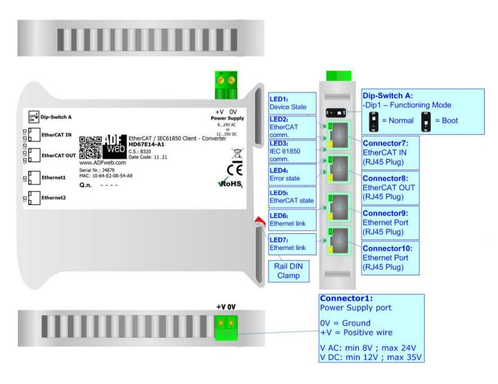
Figure 1: Connection scheme for HD67E14-A1
