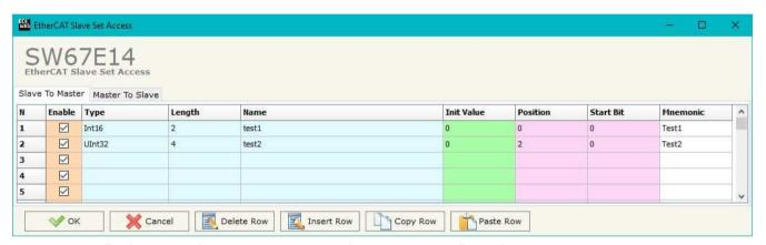
Figure 4a: "EtherCAT Slave Set Access → Slave To Master" window
