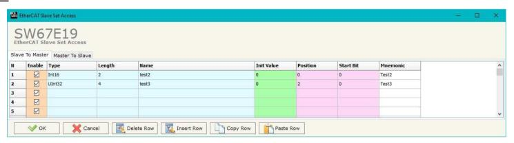
Figure 4a: "EtherCAT Slave Set Access → Slave To Master" window
