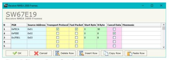
Figure 5: "Receive Frames" window
