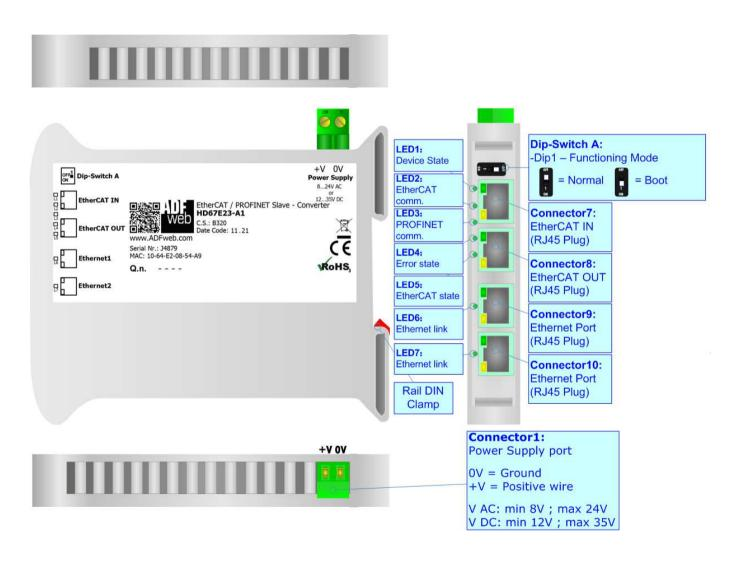
Figure 1: Connection scheme for HD67E23-A1
