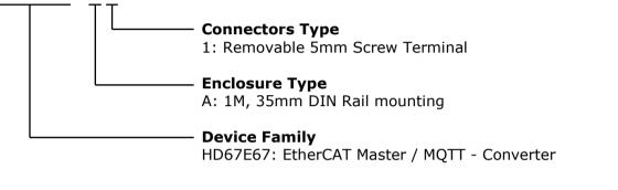
Order Code: HD67E67-A1 - EtherCAT Master / MQTT – Converter
