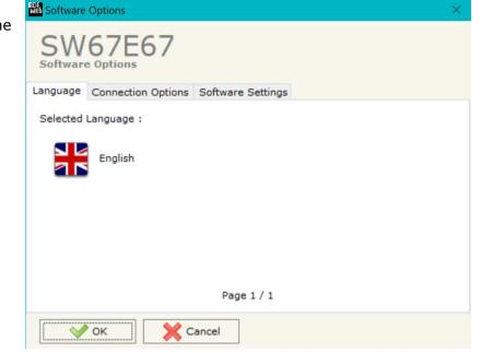
In the section "Connection Options", it is possible to check if there are some updatings of the software compositor in ADFweb.com website. Checking the option "Check Software Update at Start of Program", the SW67E67 checks automatically if there are updatings when it is launched.
